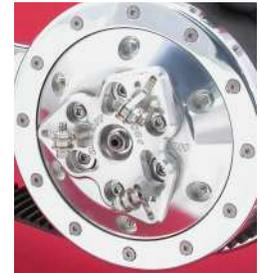
The drive shown below, with 3.35 belt, Superclutch, Bandit 3 finger lockup and 8 hole lockup cover is PN 064999
