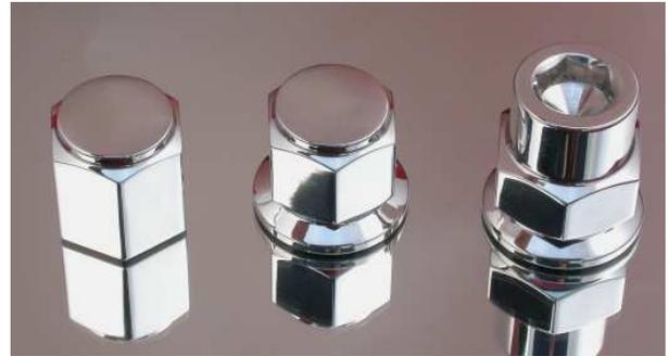
Three Sprocket shaft nuts are available, #1 at left is plated steel, standard equipment on drives where the nut is exposed. #2 Center is Stainless steel and incorporates a flange to eliminate the need for a washer. #3 on the right is also stainless and has a decorative hex broached into the end. These nuts are compatible with other belt drives.
