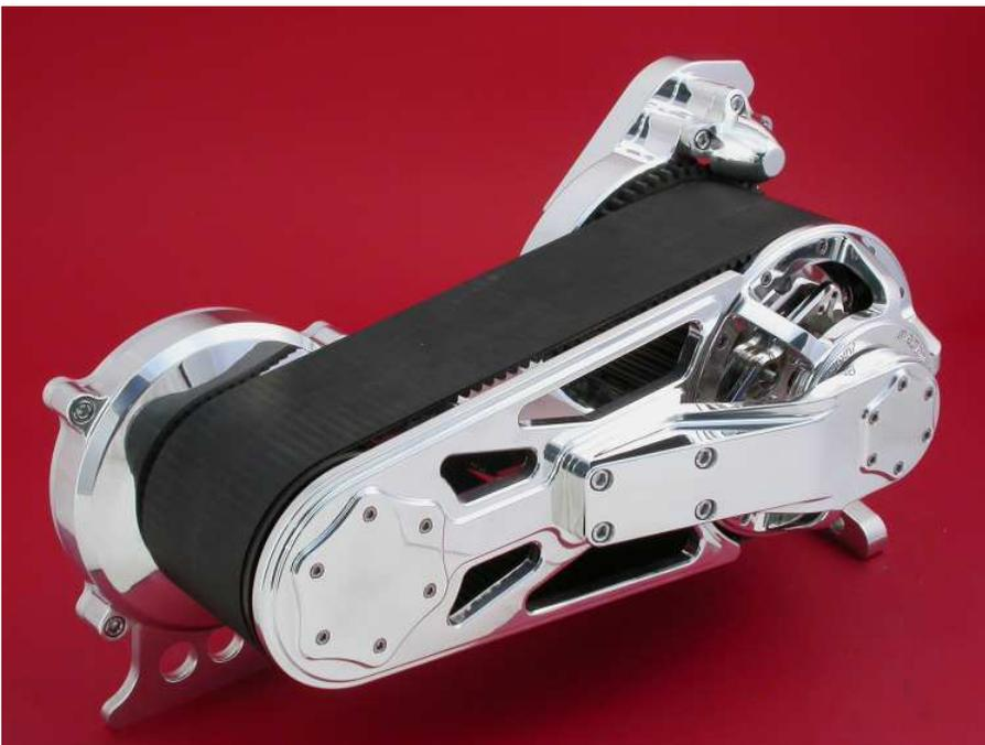
Yes, we've got it - If you just have to have the big one, here it is! All the same features as the 3.35" drive with bearing supports on a 4 inch wide belt. Go ahead, try to break this one. The lockup support covers are also available in 3 configurations, 6 hole, 12 hole and star pattern.
