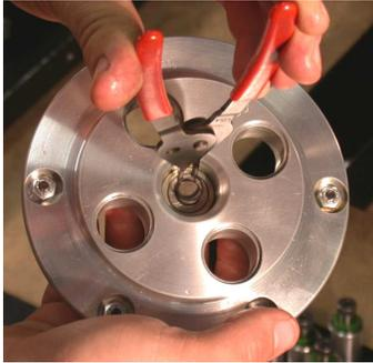
release bearing in your new pressure plate. Install the snap ring as shown, if your bike was equipped with one.
