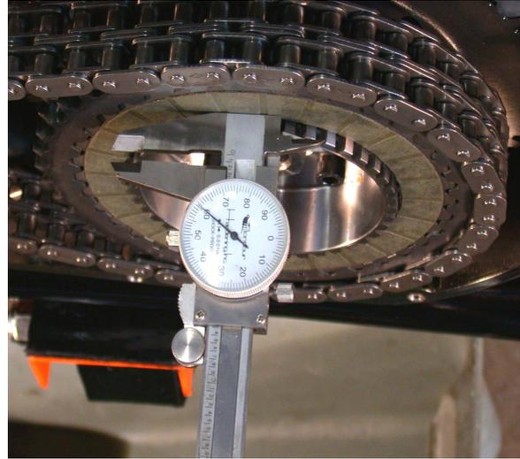
15. Installing the pressure plate: Align the timing mark on the rear face of the pressure plate with the timing mark on the face of the splined hub and install. Insert the spring cups into the pressure plate. Insert the springs into the cups, followed by the shoulder bolts. Use blue loctite. Torque to 25 lbs. (*See below for more information on spring pressure adjustment. Install shims under the springs to increase static pressure*) Also see below for clutch cable lubrication recommendation.
