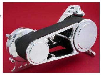
The 3.35" belt gives you enough room to put a full length oil filter under the guard. Mix and match any way you like. As shown here with geometric guard, contour cover and oil filter, PN 065135
