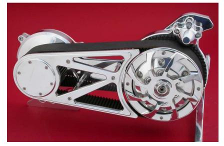
The right side drive option includes a motorplate which covers the left side of the transmission case as shown at right. This is available on all Softail Modular Motorplates.
