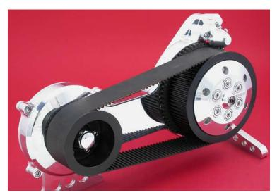
Tech note: We recommend that 2" belts be reserved for bikes with 80C.l. motors or smaller, and preferably on lightweight bikes. 2.5" belts are good up to 125 hp. 3" belts are good for just about any "street" bike. 3.35" belts will handle the monster motors, and heavy rigs. 250 hp Pro Mod drag bikes run our 2" belts with success, however, we like to be conservative in our recommendations because of the varied conditions of service encountered.
