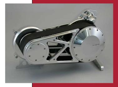
For the neglected FXR, a race quality open belt primary drive witrh all the performance and precision you expect from Bandit. Available with many options of clutch equipment, belt width (2" to 4"), outboard support, mid control shifter, with lockup, etc, etc, etc. Comes with a solid one piece motorplate to support the rubber mounted FXR engine and trans.
