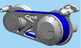
Bolt on to 1990 – 2006 Touring models, integrated shifter mount uses all stock or custom shifter components, no modifications to floorboards needed.
