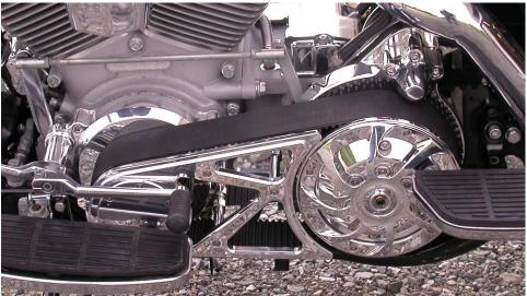
guards and pulley covers available, also available without shift linkage mount for custom forward control applications. Light lever pull, high horsepower capacity, long life clutch reduces maintenance.
